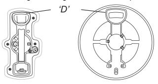
Turn the head until the 'D' matches the one on the burner base. Turn the head over and place it on the burner base. To fit the small inner burner, find the larger electrode notch in the burner rim. Line this up with the white ignition electrode and place the inner burner on the large base ring.
